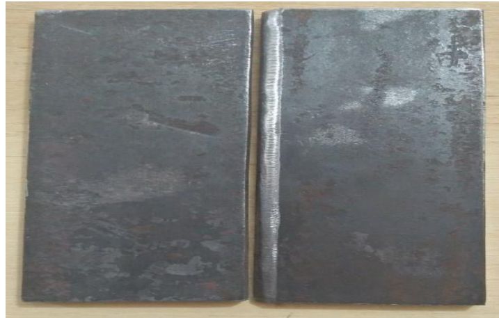
Figure 01: Two plates with V Bevel Edge
