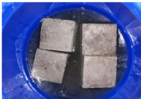
(c) Water Absorption Test
