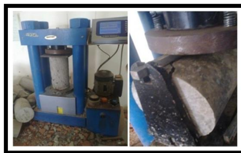
Figure 4: Compression and Split Tensile Test on CTM
