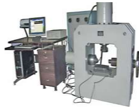
Figure 4. YZW30 computer-controlled rock stress direct shear apparatus
