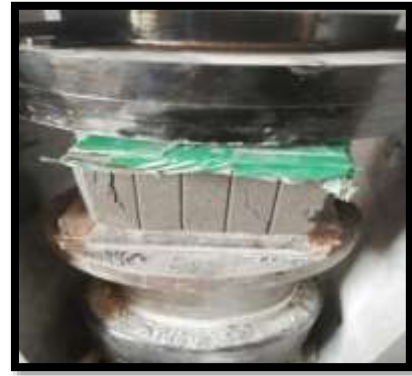
Figure 2. Compressive Strength Test on Brick
