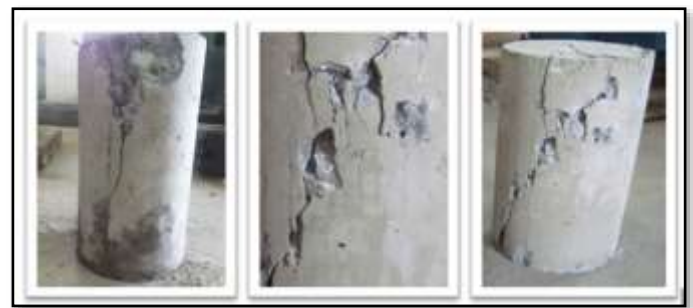
Figure 5. PC Mix Cylinders after Compressive Test
