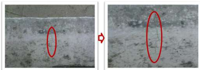
Figure 9. FC Mix Beam after Flexure Test
