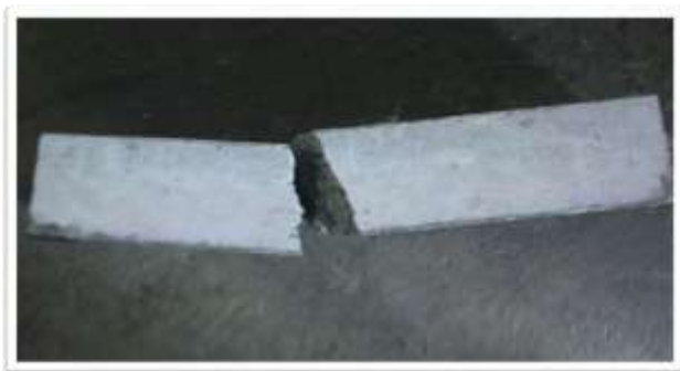
Figure 8. PC Mix Beam after Flexure Test
