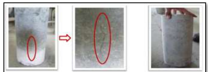
Figure 6. FC Mix Cylinders after Compressive Test
