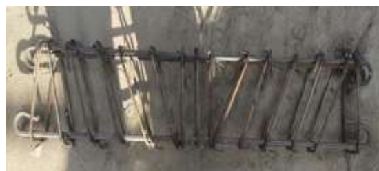
Steel reinforcement at 60° Angle
