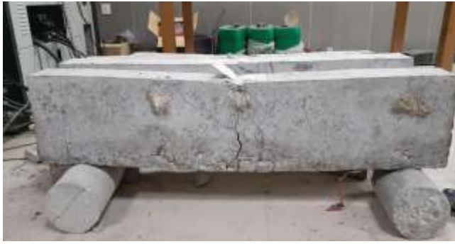
Cracking of Beam at 60° Angle
