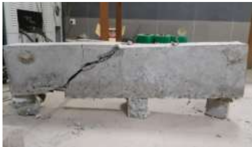
Cracking of Beam at 30° Angle
