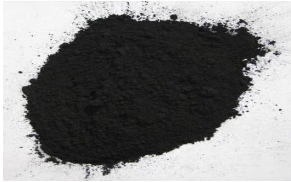
Figure 2 Toner Waste Product Used for Soil Stabilization
