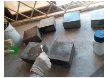
Applying Copper Chloride Acid Solution on concrete cubes
