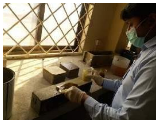
Applying Ferric Sulfate acid stain to cube sample
