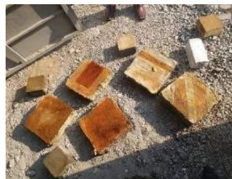
Application of different stain solutions to concrete cube and slab samples
