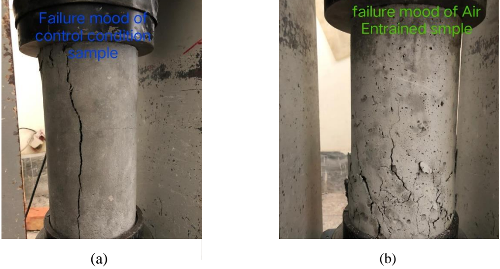
Fig. 7 (a) Failure mode of C.C.S after 28 days (b)Failure mode of A.E.S after 28 days
