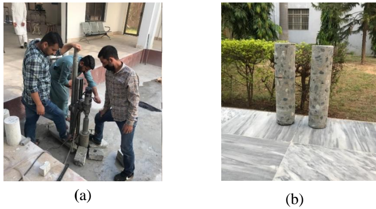
Fig. 8. Core cutting for Freeze-thaw test
